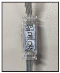
The P50T, 4-wire Pebble is the single-sided version Rainmin has manuafactured since 2019, without the magnifed lens & deeper body of the P50L & P50H versions.
